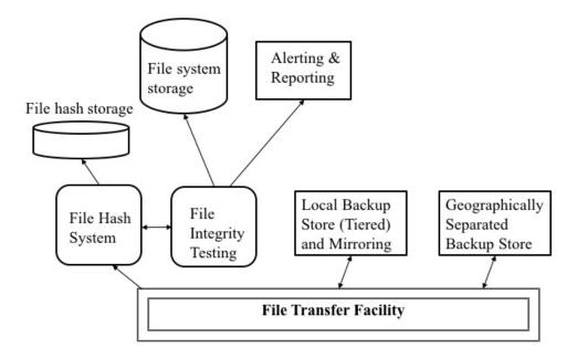
Figure 1. Data Integrity Building Block high-level architecture
