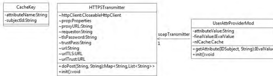
Figure 10.4 NextLabs PIP Plugin cCass Diagram
