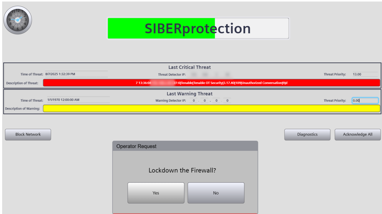
2332 Figure 4-169: SIBERprotect HMI indicates threat detected
