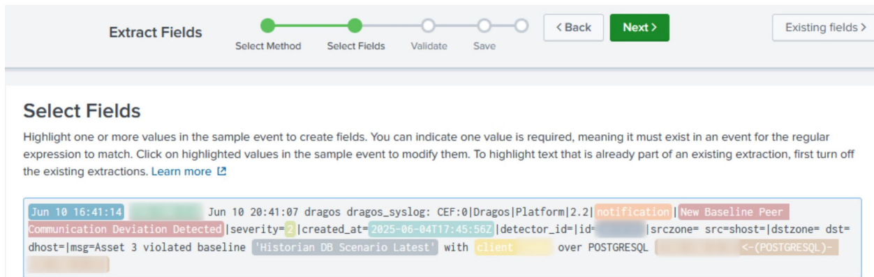
2042 Figure 4-100: Same extracted fields as before, no more error after increasing Regex limit values
