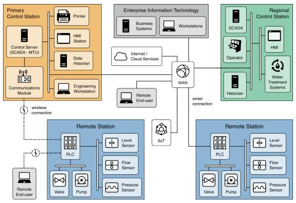
Figure 1 WWS Reference Architecture
