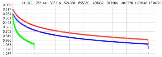
Client time vs. bytes sent, bytes acknowledged, bytes in acknowledgments. Curve shows packet pacing from our new user-level congestion-control library.
