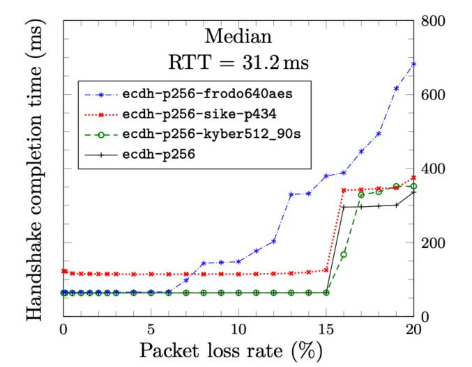
Measured effect of packet loss rate and connection latency on TLS handshake time for various PQ KEMs and signatures using a network emulation framework
